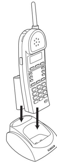
1. Charge the battery pack in the battery port at the back of the charger for a minimum of 30 minutes.
