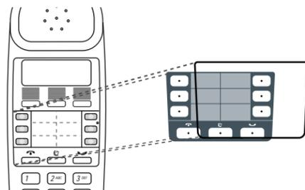
1. Remove the plastic lens and handset card from the handset.
